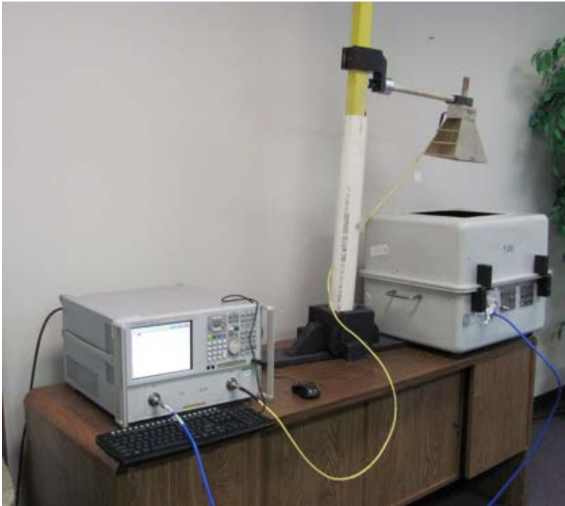
Figure 5. High Frequency Test Configuration Photograph – Above 6 GHz Testing
