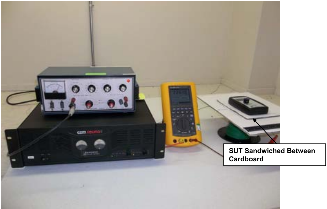
Figure 9. ELF EMR (Magnetic Component at 60 and 300 Hz) Test Configuration Photograph
